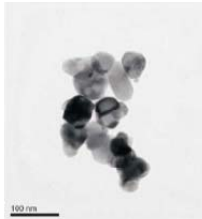
Zirox-TZY-DW dispersion particle size Image @ 20 nm & 100nm
